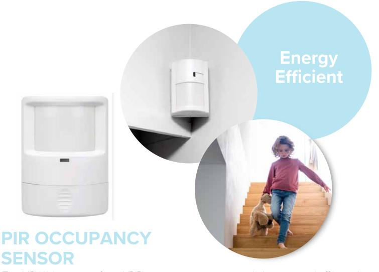
The MPW-V passive infrared (PIR) occupancy sensors turn lighting on and off based on occupancy and ambient light levels. The light level feature keeps lights from turning on if the ambient light level is sufficient. The sensors can be configured to turn lighting on, and hold it on as long as PIR technology detects occupancy. After no movement is detected for the selected time delay, the lights switch off.
