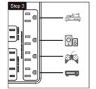
Plug in TV peripheral electronics (AV receiver, DVD player, etc.) into the outlets labeled "AUTOMATICALLY SWITCHED OUTLETS".
