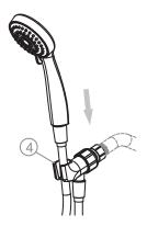
Step 5: Turn on the water to check for leaks and gently tighten any coupling if you notice water dripping. Do not over tighten.
