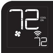
When you see the thermostat's idle screen, it means you are connected. You can now replace the Décor-snap cover.
