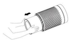
3. Take out the preinstalled HEPA filter.
