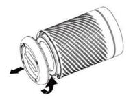
2. Rotate the base counter-clockwise.
