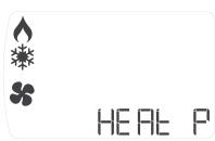
**NOTE:** If you have a heat pump system, press the center button to select. Greenlite  $Airz^{TM}$  will now ask you to confirm your valve type. Use the up and down arrows to toggle between O & B Valves, press the center button to select.
