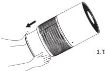
3. Take out the preinstalled HEPA filter.
