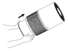
5. Install the new HEPA filter back in the unit.
