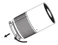
2. Rotate the base counter-clockwise.
