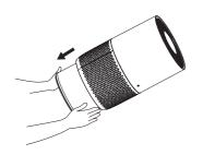
Remove old filter and replace with only a Greenlite G-Pure-15W HEPA filter.
