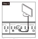
Plug the TV into the outlet labeled "CONTROL OUTLET"
