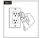
Plug the power strip into a grounded wall receptacle.
