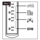
Plug in TV peripheral electronics (AV receiver, DVD player, etc.) into the outlets labeled "AUTOMATICALLY SWITCHED OUTLETS".
