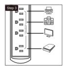
Plug in TV peripheral electronics (Printer, monitor, speakers, etc.) into the outlets labeled "AUTOMATICALLY SWITCHED OUTLETS".
