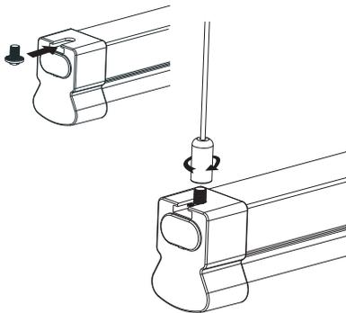
3. **Attaching the chain to the ceiling** Hang the fixture body by placing one chain set over each hook that has been installed on the ceiling. Adjust chains to level light. Hang lamp low enough so that you are able reach the on and off button. The lamp should hang at least 3 inches from the ceiling or maximum height from floor to lamp is 78.75 inches.
