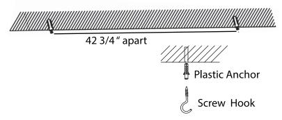
3. Attach the chain to the two hooks mounted on the mounting surface.
